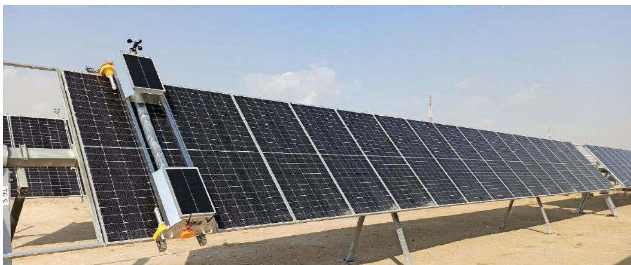
Figure (1): Waterless PV Panel-Cleaning Robot that is Being Tested by a Government Entity in Dubai Desert
